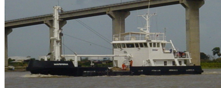
Boeienlegger en survey vaartuig Marwina ; coastal survey length 35m, width 7m, draft 1.80m
