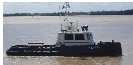
Pasisi ; river surveys length 14.40m, width 4.73m, draft 1.80m
